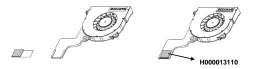
Figure 4-44 Apply new thermal pad on the fan
